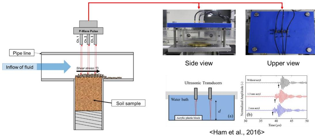
Fig. 1 EFA set-up
